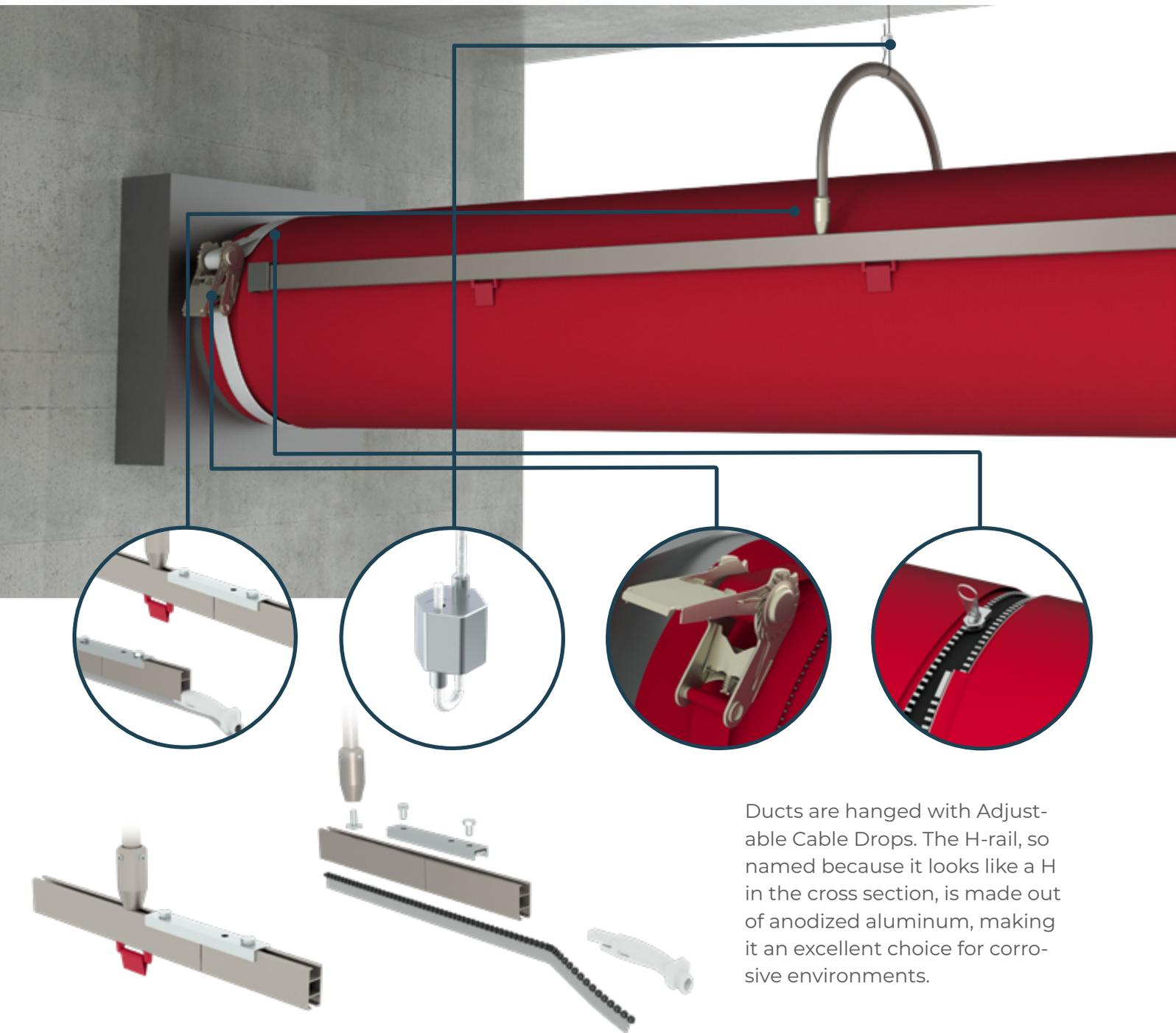
Ducts are hung with Adjustable Cable Drops. The H-rail, so named because it looks like a H in the cross section, is made out of anodized aluminum, making it an excellent choice for corrosive environments.
