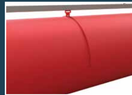
All-in-One Support added to a Type 8 suspension in an external pocket.
