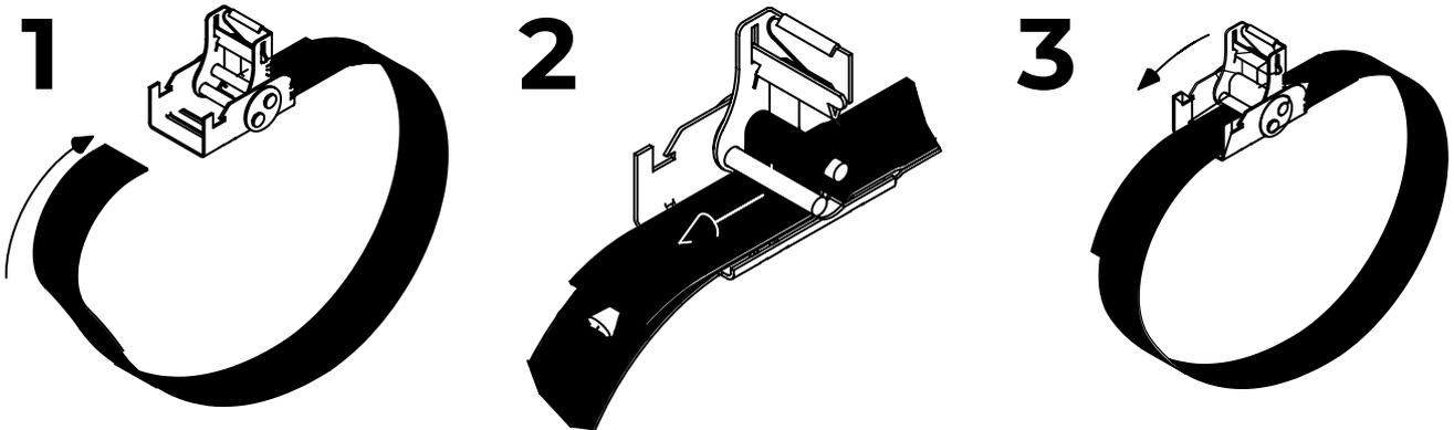
Part ID (18) Duct  $\varnothing \geq 510$  mm [20"]
