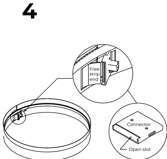
Put connector on the aligned strip end with the open slot towards the free strip end
