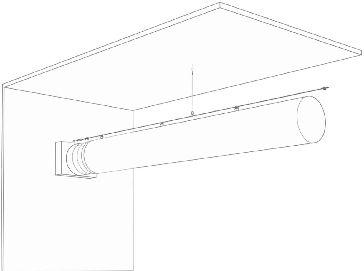
Type 01 cable suspension is compatible with classic, All-in-One, and Internal 360° Hoops ducts.
