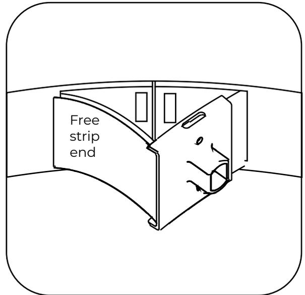
Hold the connector and the free strip end together and push until both strip ends are aligned
