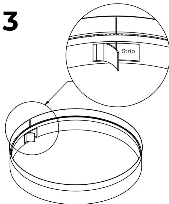
Align one end of the strip with the seam line
