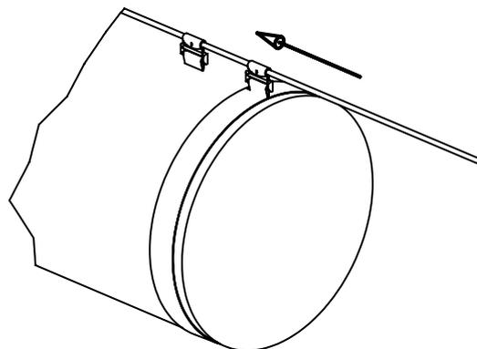
\* Secure duct when fully extended with cable locks as slide stops to ensure best aesthetics
