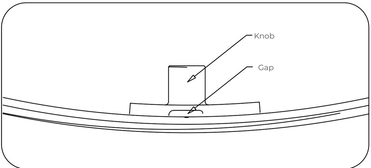
Using the knob, slide the connector and make sure the gap between both strip ends is in the center of the connector
