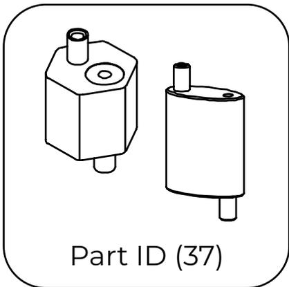
Adjustable cable lock for vertical hangers
