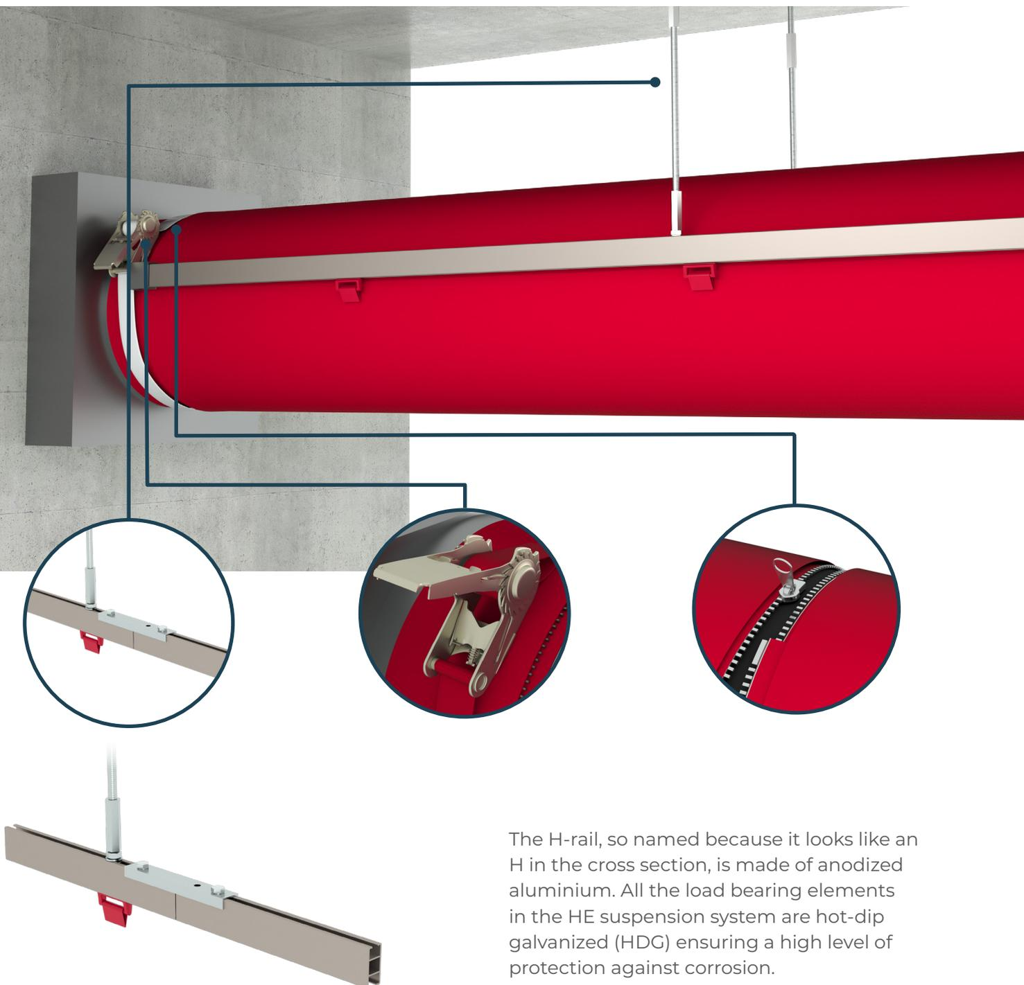
The H-rail, so named because it looks like an H in the cross section, is made of anodized aluminium. All the load bearing elements in the HE suspension system are hot-dip galvanized (HDG) ensuring a high level of protection against corrosion.
