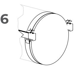
Fix end lock by turning bolt clockwise
