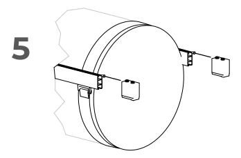
Secure duct by inserting end lock
