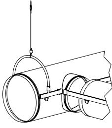
Bottom aligned branch with extended strap length
