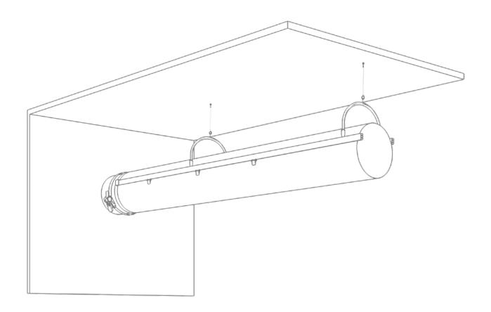
Type 13 is a suspension method for round fabric ducts, which makes use of two H-Rails joined by a factory bent aluminum hoop. Each hoop requires only a single point connection to the structure. This double rail suspension method prevents the duct from twisting that may occur with unbalanced distribution, while maintaining the simplicity of install of a single-point suspension method. Type 13 is not compatible with shape retaining hardware (All-in-One, Internal 360° Hoops).
