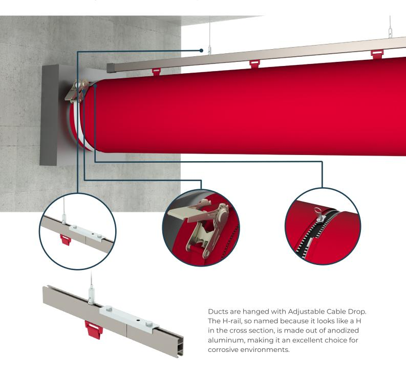
Example of duct system configuration
