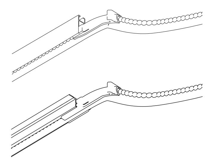
The RapidSlider allows you to install fabric duct with a T-Rail or H-rail suspension system even faster. The specially designed feeder makes it easy to slide any length of duct continuously through the suspension rail with little or no additional labor or equipment.
