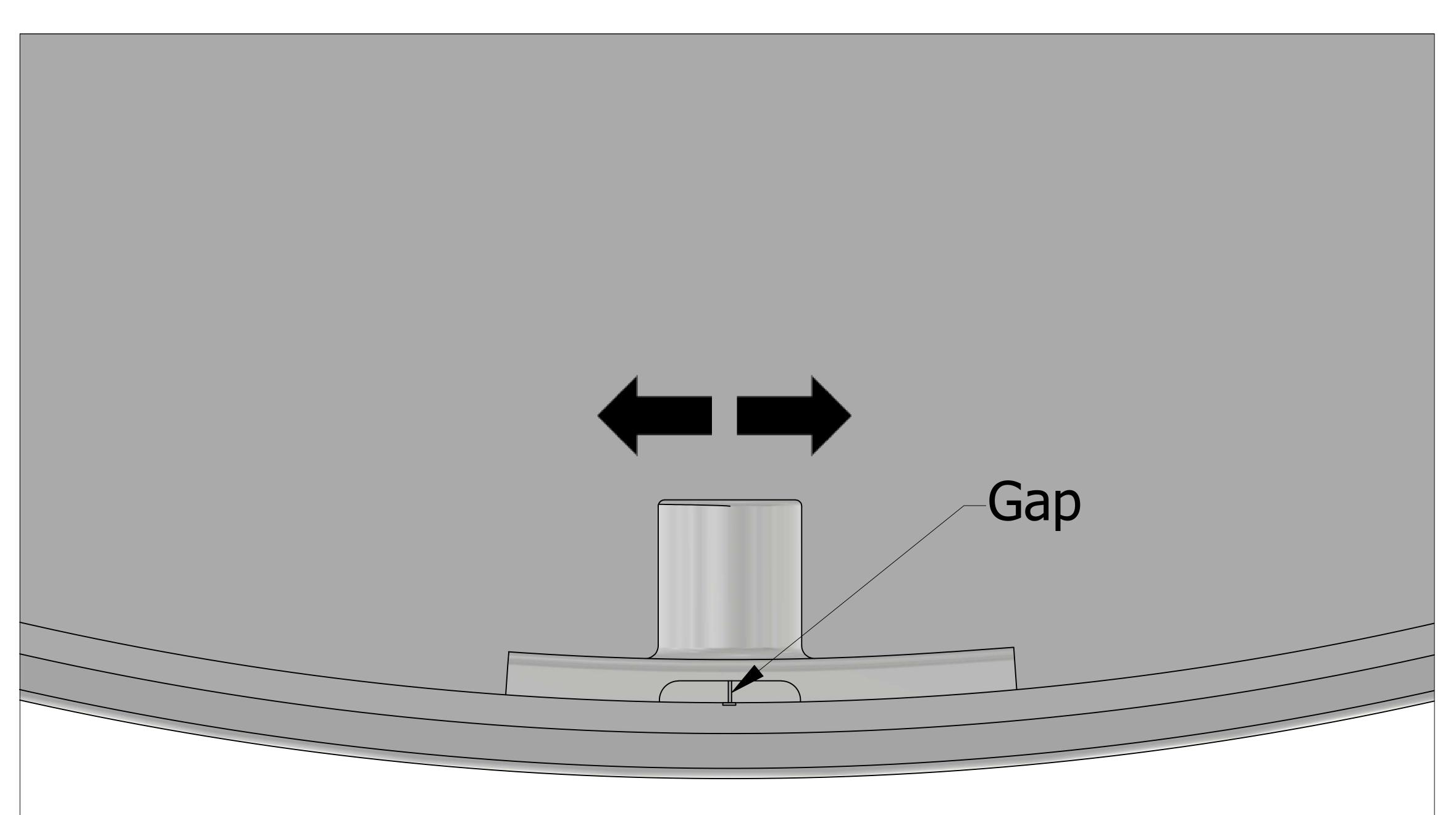
5.3 Using the knob slide the connector and make sure the gap between both strip ends is in the center of the connector
