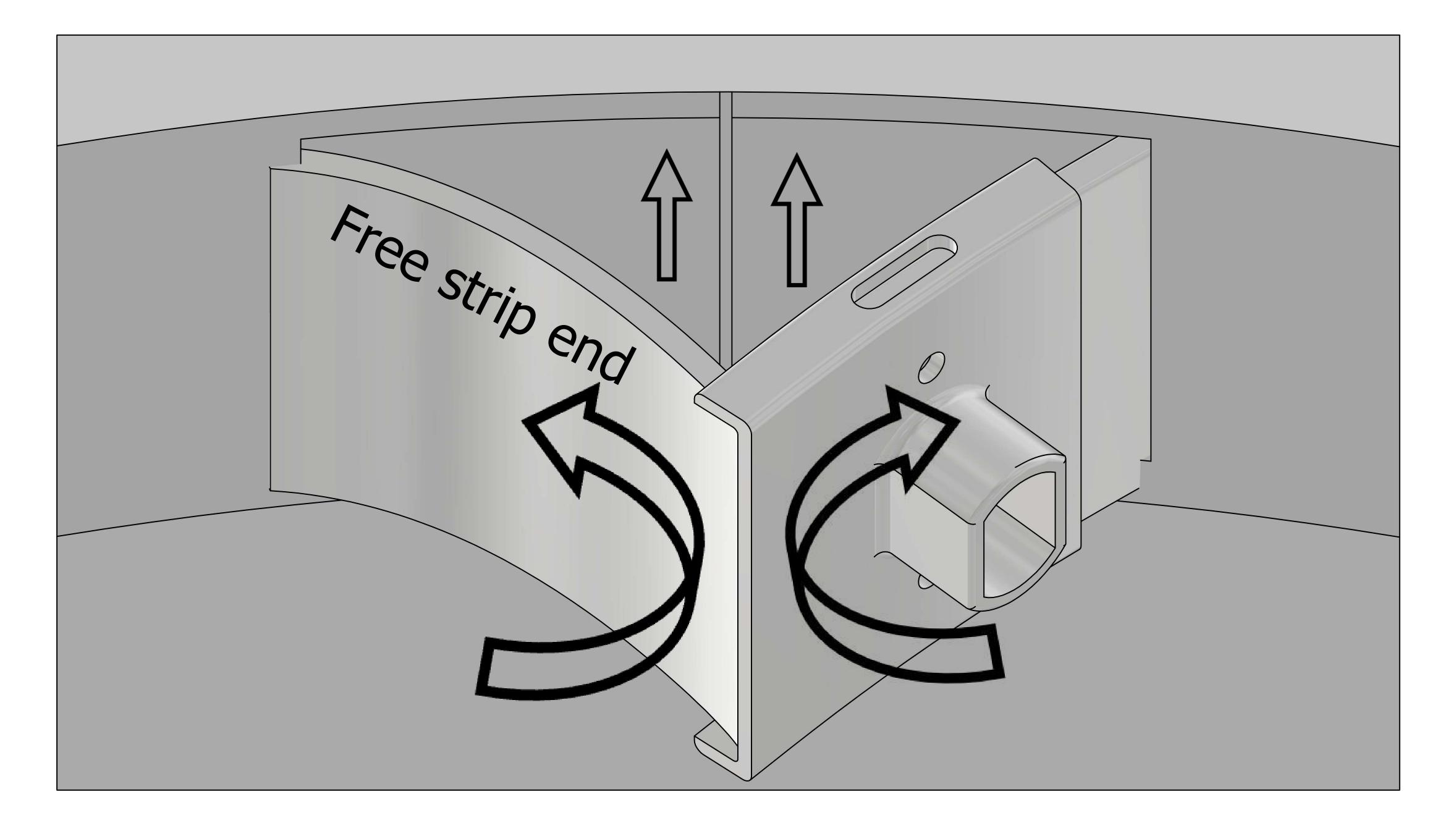
5.2 Hold the connector and the free strip end together and push until both strip ends are aligned
