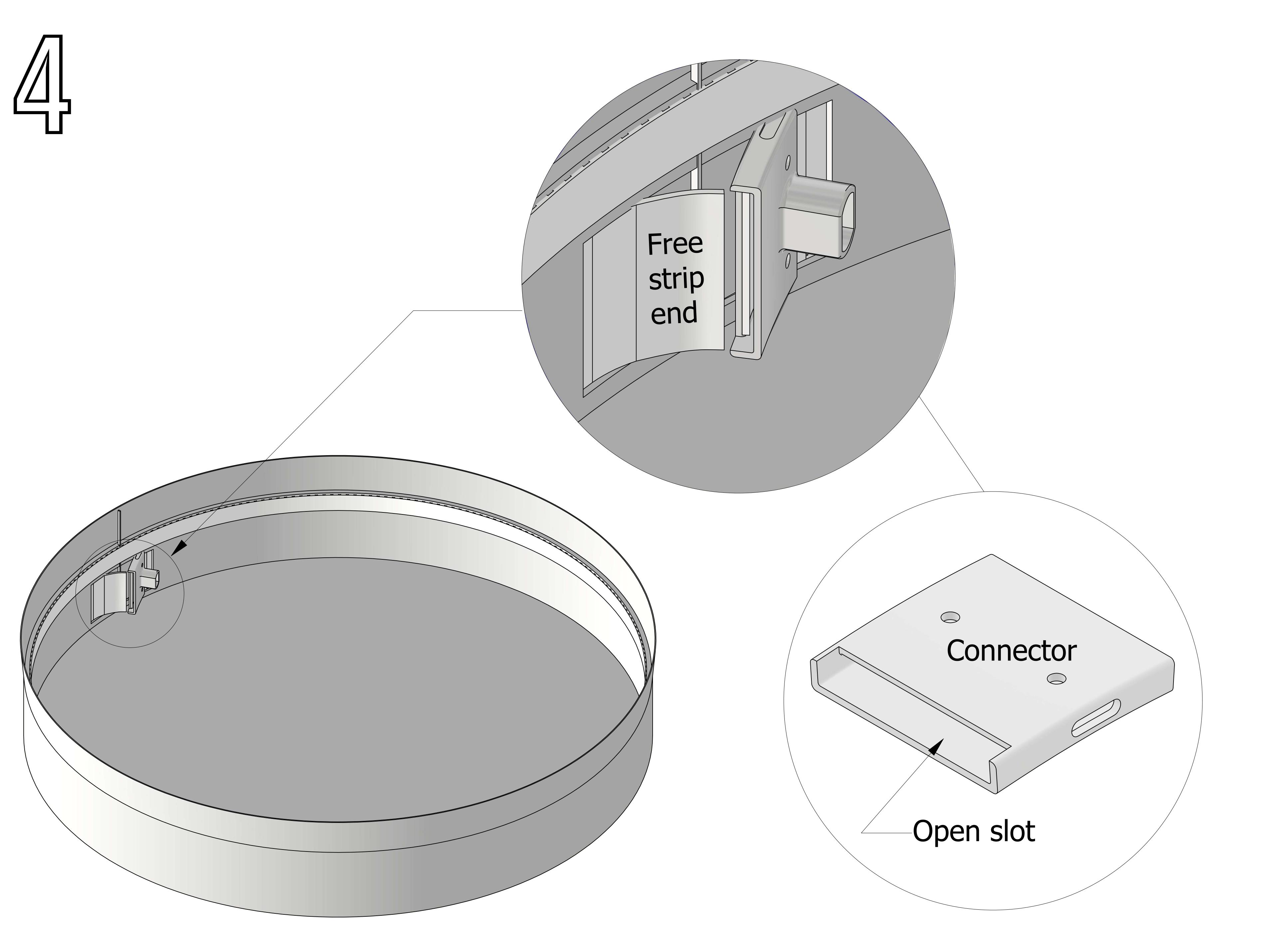
Put connector on the aligned strip end with the open slot towards the free strip end
