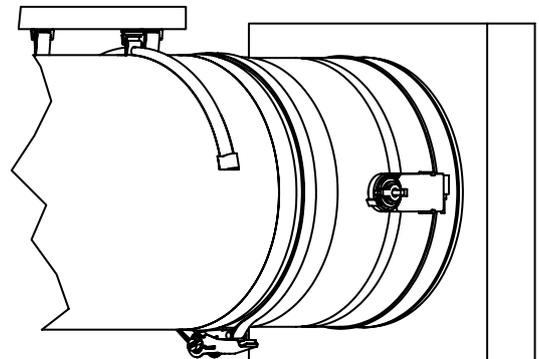
In case actuator position needs to be replaced after delivery, please contact FabricAir for instructions.
