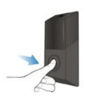
Insert speed controller wire jack fully into the connection port until it clicks into position. Secure in place with a plastic locking nut located on the speed controller wire.
