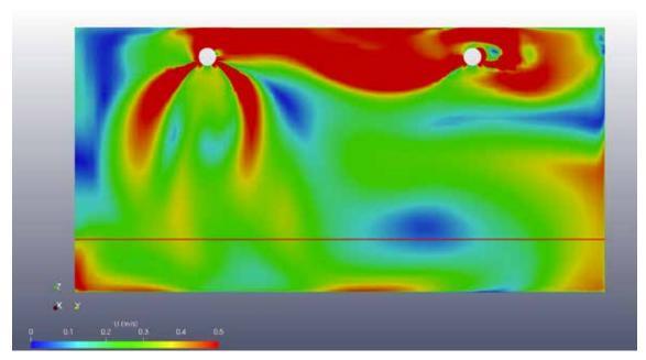
**Figures 4** below shows how air is discharged from the ducts via the SonicFlow<sup>™</sup> flow model at the 4:00 and 8:00 o'clock positions on the duct.
