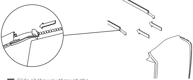
**3** Slide all the way through the feeder to install
