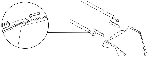
**3** Slide all the way through the feeder to install
