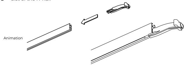
2 Insert the RapidSlider into the feeder
