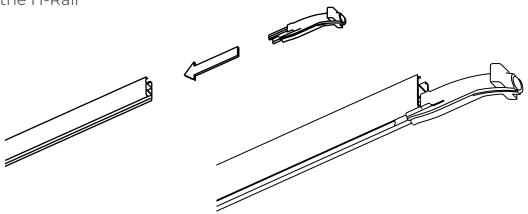
2 Insert the RapidSlider into the feeder
