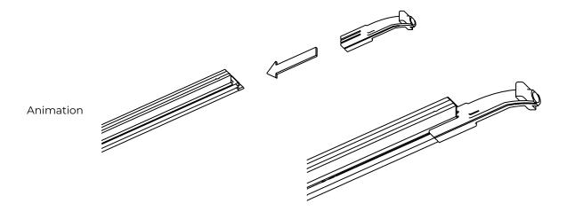
2 Insert the RapidSlider into the feeder
