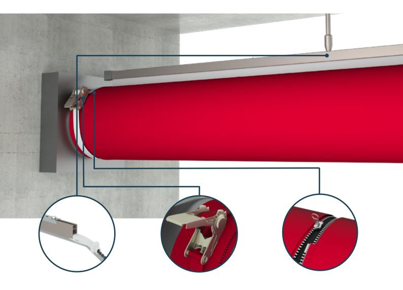
The ducts hang by a keder type bulb edge. The H-rail, so named because it looks like a H in the cross section, is made out of anodized aluminum, making it an excellent choice for corrosive environments.
